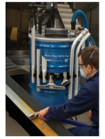
A technician uses a Heavy Duty HEPA Vac to perform scheduled maintenance on a pulverizer.
