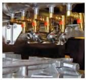
A combination of Model 6013 High Velocity Air Jets and Model 6042 Adjustable Air Amplifiers dry this engine casting.
