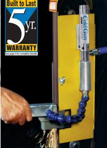
The Model 5215 Cold Gun keeps the part cool to the touch and prevents discoloration.
