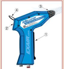
Pressing the full finger, short throw trigger (1) activates the static eliminating ions and airflow. Proper or improper functionality is indicated by a green or red LED (2). The non-maring nozzle (3) provides quiet performance and OSHA compliance. A hanger hook (4) is included to keep the Intellistat conveniently stored.
