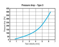
Typical pressure drop of a two-stage system type 3.
