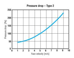
Typical pressure drop of a two-stage system type 2. Figures are valid for face velocity at operating point and for clean filters.
