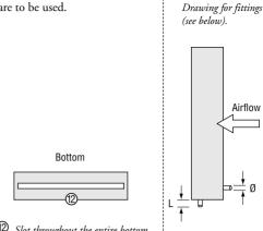
D Slot throughout the entire bottom for use with separate housing/tray.
