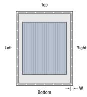
Hole configurations in flanges are delivered according to Eurovent, DIN 24193, Norsok or other trade, national or international standards (specify standard). Hole configuration according to individual requirements are also delivered (specify drill pattern and hole diameter, provide a drawing).
