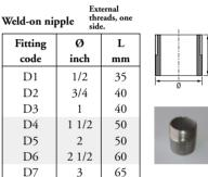
Bushing according to DIN 2986, nipples DIN 2982, material 316Ti (AISI 316Ti, DIN 1.4571), witworth thread according to DIN 259.
