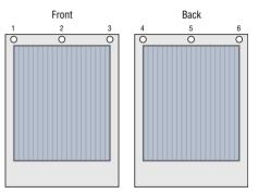
Code for cable output position, put CO before the position number (1-6) e.g., CO1. **Only one position is possible!**
